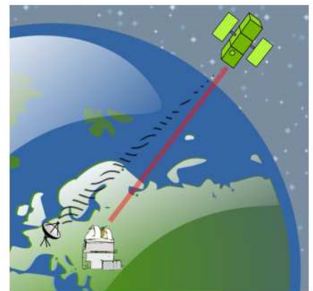
Figure 1: mission configuration. Single (entangled) photons are sent from the Vienna telescope to the receiver on board of the NanoBob cubesat. Satellite control and data transmission is done by conventional radio communication.
