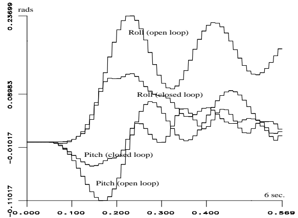
Figure 5: Roll and pitch errors during arm motion
