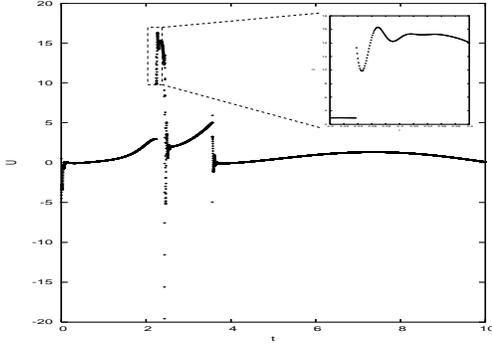
Fig. 3. The control law applied to  $\theta_1$  during the first round.
