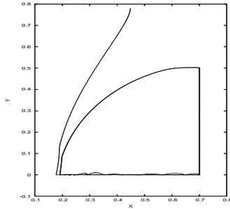
Fig. 4. The variation of the end-effector coordinates using the rigid controller when the stiffness matrix is defined by  $K = \text{diag}(5000N/m, 5000N/m)$ .
