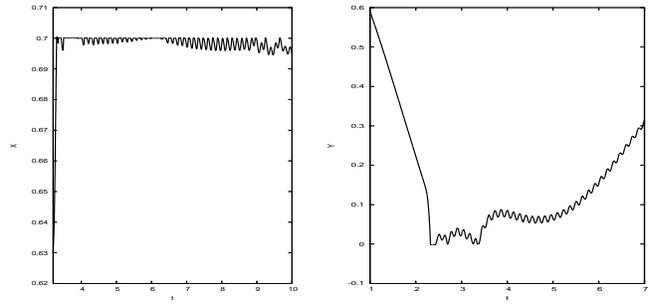
Fig. 5. The variation of the end-effector coordinates using the rigid controller
